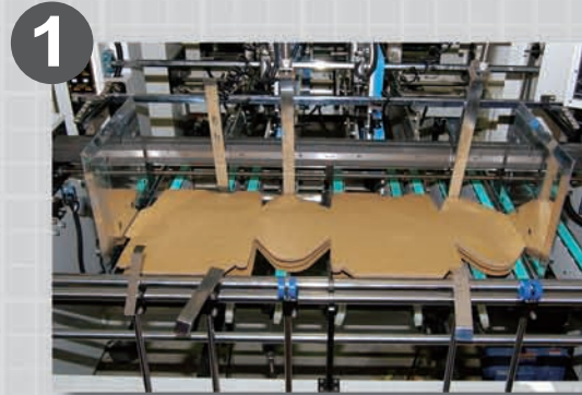
1 給紙部 Feeder Section 自動定位側擋板、撐紙桿電動移動、氣壓式出紙刀使彎曲紙張出紙順暢。操作簡單，設定快速！ The side guides and supporting shafts at the feeder section are automatically and conveniently adjustable by motor; With Air Pressing Feeding knives to achieve a smooth feeding, even when blanks are curved and transformed on the shapes.
