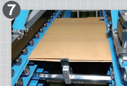
7 壓著部收葉矯正裝置 Alignment Device at Trombone Section 紙張在壓著部經矯正後進入輸送機，避免魚尾開叉。 The cartons enter the Conveyor section after alignment at Trombone section which is another effective solution to reduce the fish tail problem.
