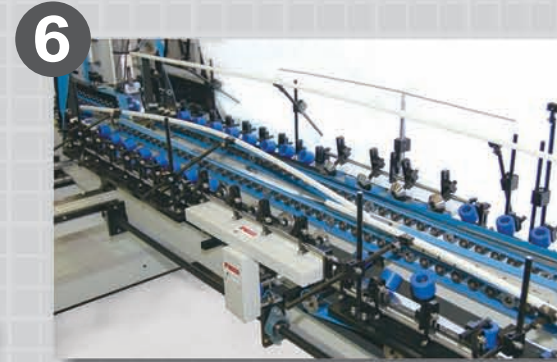
6 本折部 Final Folder Section 強力的折線結構，平順的折合動作，能更精準地折合成型，減少滄浪和魚尾公差。 It enforces the folding strength to form cartons precisely and offers a great help to avoid the possibility that the groove lines between flutes become the folding lines and to reduce the problem of fish tails.
