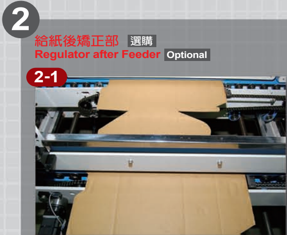
2 給紙後矯正部 選購 Regulator after Feeder Optional 2-1 伺服矯正裝置 Servo Regulator Section by Chain after Feeder 使用鏈條導正推齊，使紙張不歪斜，正確的前進。 By using the chains to guide and push the blanks to move correctly without slanting problem for the next procedures.
