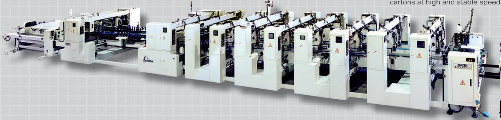
4 四角裝置 選購 4-Corner Back Finger Attachment Optional 四角盒尺寸設定簡單容易，後踢動作精確穩定快速。 With this device, it is easy to set up the 4-Corner cartons. With the unique design for back finger attachment to produce 4-corner cartons at high and stable speed.
